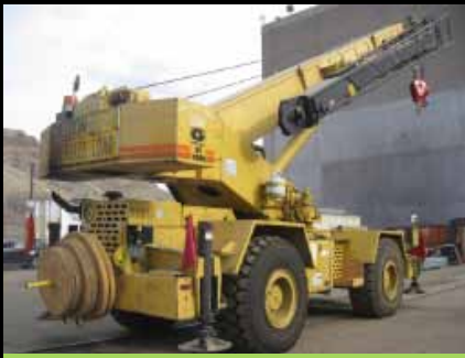
1988 GROVE RT700B 35-TON ROUGH TERRAIN CRANE
