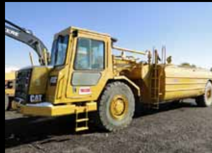
CATERPILLAR 613C WATER WAGON, 5,000 GALLON CAPACITY
