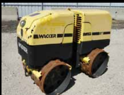
2006 WACKER RT TRENCH COMPACTOR, COUNTY UNIT
