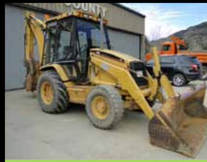
CATERPILLAR 426C 4WD LOADER/BACKHOE, EXTENDAHOE, COUNTY UNIT
